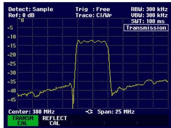
The transmission calibration remains valid until the Center Frequency or the Span is changed on the R&S FSH3. **Track Gen Uncal** is displayed in the top right-hand corner of the screen when calibration is no longer valid.
