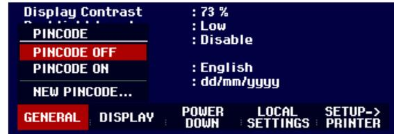
Use the Rotary knob or the Cursor keys to select the PINCODE... menu item and press the ENTER key. The selection box with the PIN code settings is opened.
