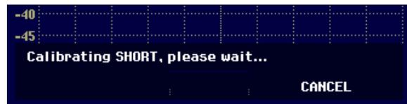
When SHORT calibration is over, the R&S FSH3 prompts the user to terminate the measurement plane with a 50-Ω LOAD.
