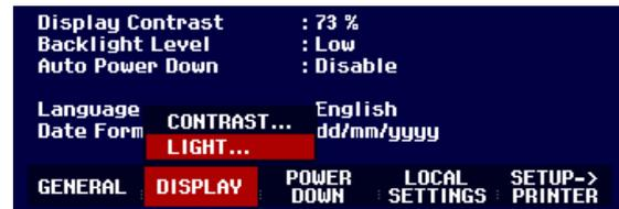
The BACKLIGHT sub-menu for the lighting level opens. The level can be set to HIGH, NORMAL and LOW.
