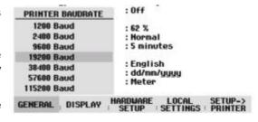
Note: If the serial/parallel converter (R&S FSH-Z22) is used to control a printer with a parallel interface, set the RS-232-C interface to 38 400 baud.
