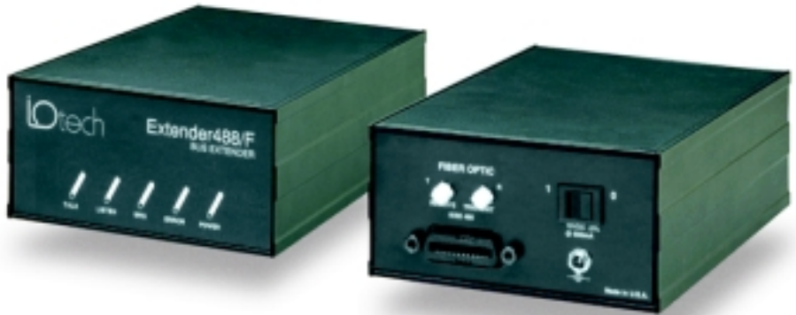
Extender488/F enables instruments to be located up to 4,000 feet from host IEEE controller
