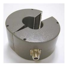
The F-130A-1 is used for BCI testing in accordance with automotive specifications like SAE J15447 as well as diagnostic bulk current testing up to 400 MHz. The useable frequency range is 10 kHz to 400 MHz with a typical insertion loss of 6 dB or less from 1.5 MHz to 400 MHz. The CW input power rating is 100 watts for a duration of 30 minutes.
