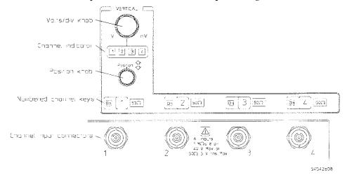
When you press a numbered channel key on the front panel, the vertical menu that corresponds to the key you pressed is displayed on the right hand portion of the screen. The vertical menu and menu map are shown below.
