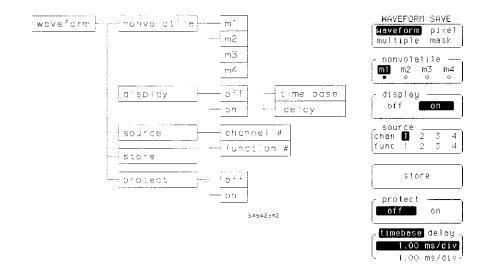
A waveform memory consists of a single waveform record, including the horizontal and vertical scaling parameters. The scaling parameters allow measurements on previously stored waveform and function data. Also, you can set the x and y markers on stored waveforms when they are displayed on the screen.
