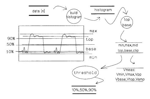
The oscilloscope calculates the 10, 50, and 90 percent thresholds
