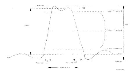
Pulse parameters the oscilloscope measures
