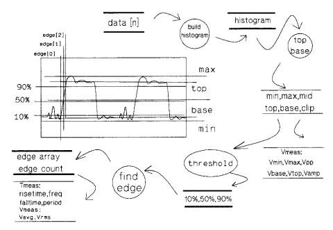
Thresholds are used to determine edges
