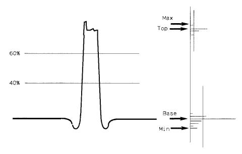
Some measurements are made from the histogram
