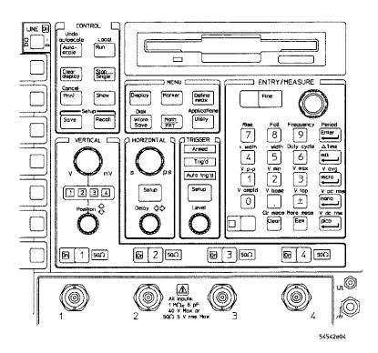
There are two types of keys: front-panel keys and softkeys. A front-panel key has text or numbers printed on it, or it is blue in color. Softkeys are to the right side of the display, and the labels for the softkeys are displayed on the screen next to each softkey. These labels are referred to as menus, and which menu is displayed depends on the front-panel key you press. Not all front-panel keys cause softkey menus to display on the screen.
