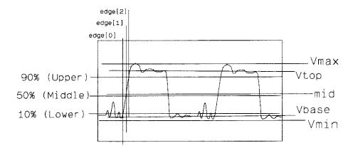
Waveform definitions used to make voltage measurements
