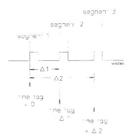
When the sequential softkey is set to on, the screen is cleared and the oscilloscope is placed in the stopped state to allow selection of the acquisition parameters (number of points and segments). The sample rate is set by the time/div knob as per table 4-2.
