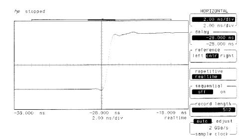
To see the raw data points, use the repetitive mode or turn off the interpolator in the real-time mode.
