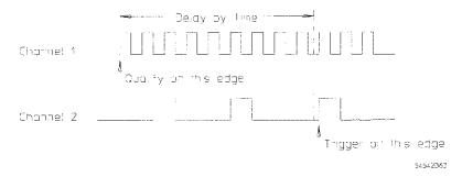
Figure 5-12 shows a delay-by-events timing diagram. You may notice that the qualifying event is channel 1, and the trigger event is channel 2. By changing the number of events, you can consecutively look at pulses in a pulse burst without the effects of jitter. After the number of events are counted, the scope triggers on the edge number you select.
