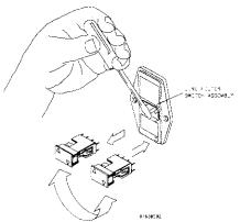
Removing and installing the fuse module.
