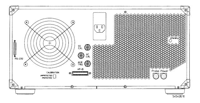
Rear-panel of the oscilloscope
