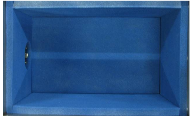
Internal anechoic walls
