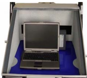
Internal anechoic walls
