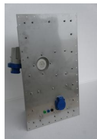
Line filter with I-LED lighting option incorporated
